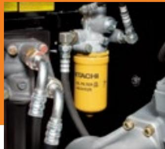
■ Engine oil, fuel and hydraulic pilot oil filters are all located on the same side at ground level for easy servicing.
