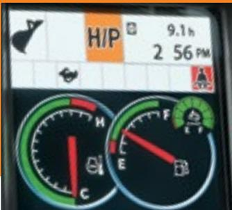
■ Easy-to-navigate LCD monitor issues scheduled maintenance alerts and diagnostic information. Additionally, the hydraulic temperature gauge on the monitor screen helps prevent downtime.
