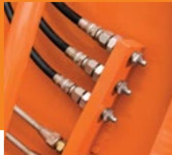
■ Centralized lube banks place greasing zerks within easy reach, making greasing less messy and time-consuming.
