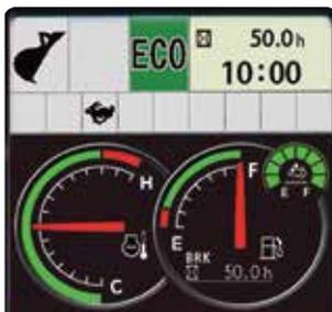
Checking DEF fluid level through Multi-function monitor.
