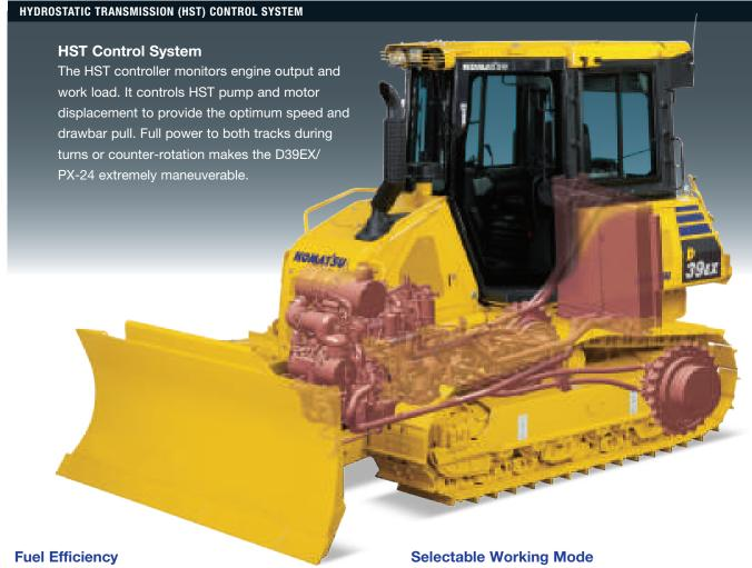
The efficient HST control system can reduce fuel consumption.
